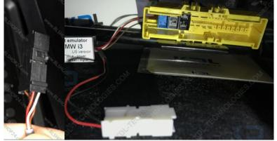
If Seat Emulator comes with wire pins then mount this original plug on our seat mat emulator wires in the same wire order. To remove plug, terminal clips should be pushed in slightly while gently pulling the wire for easy removal. Reconnect the plug now with the seat mat emulator attached to the original socket.
