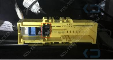
3) Now locate a small black 4 prong rectangle Plug with 3 wires: WHITE, RED & BROWN as in picture below. Disconnect original seat mat plug.
