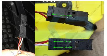
If Seat Emulator comes with wire pins then mount this original plug on our seat mat emulator wires in the same wire order. To remove plug, terminal clips should be pushed in slightly while gently pulling the wire for easy removal. Reconnect the plug now with the seat mat emulator attached to the original socket.
