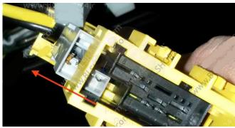
4) Use a little screwdriver to remove (red&black) wires from the plug and replace it by the emulator wires. For US spec with white&blue wires replace - white with red & blue with black.
