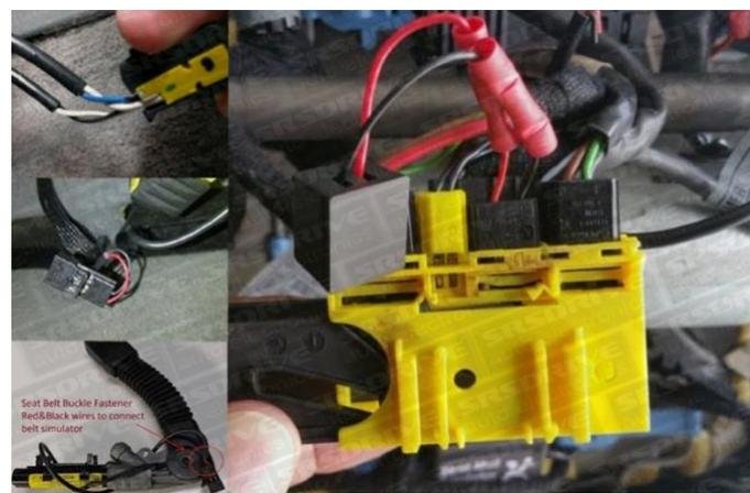
4. Disconnect it and mount this original plug on our seat mat emulator wires in the same wire order red-red & black-black or red-white & black-blue. To remove plug, push in terminal clips slightly and gently pull out the wires.
