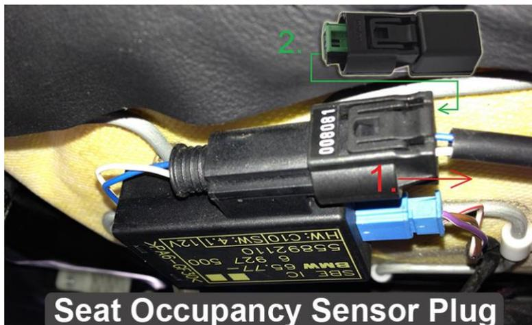
3. Turn and detach this box from the seat if needed and replace the old plug with our bypass plug. There is no need to remove the seat.
