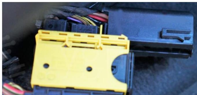
3. unlock and open connector and locate small black seat belt plug with red&black (for some US spec white&blue) wires.
