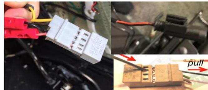
**5)** Done! - Continue to **PART 1, STEP 5**. Make sure that all plugs and wires especially Seat belt Red&Black and Pre-tensioner Grey & Green wires are connected and contacting properly!
