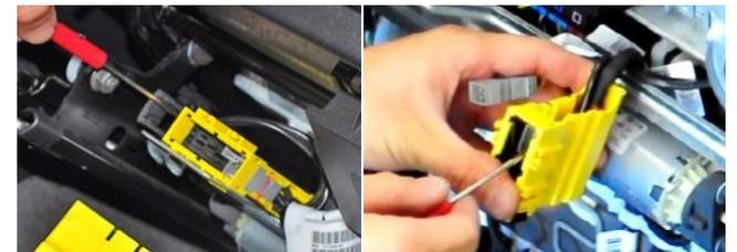
**4)** Remove original wires and replace it with seatbelt bypass wires. To remove wires, terminal clips should be pushed in slightly while gently pulling the wire out.
