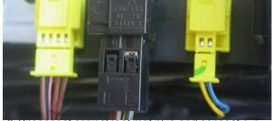
Disconnect original seat mat plug and connect our seatbelt bypass.
